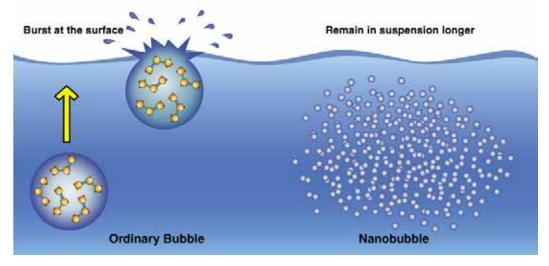
Ozone ( $O_3$ ) filled Nano-Bubbles generated by the ZERO<sub>3</sub> system provide extended cleaning effectiveness by being less likely to rise to the surface.
