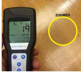
To measure how well cleaning protocols and products work, many professionals use ATP (Adenosine Triphosphate) meters to evaluate "Before" and "After" cleaning results.
