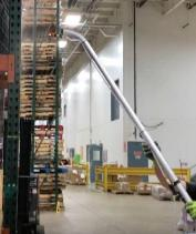
Easily sprays disinfectant solution via 25 foot hose.
