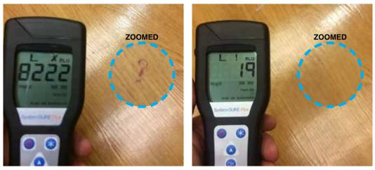
To measure how well cleaning protocols and products work, many professionals use ATP (Adenosine Triphosphate) meters to evaluate "Before" and "After" cleaning results.
