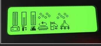
Operators quickly see bubbles on LCD display when Suds system is in operation. 6 total bubbles for "Single Dose" and 12 total bubbles for "Double Dose".
